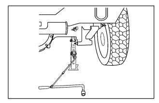
**Rear Tire Flat:** You will need to use the jack handle and both jack handle extensions. Attach the wheel wrench to the jack extensions. Attach the jack handle to the jack. Align the jack under the rear axle. Turn the wheel wrench clockwise to raise the vehicle. Raise the vehicle far enough off the ground so there is enough room for the spare tire to clear the ground.
